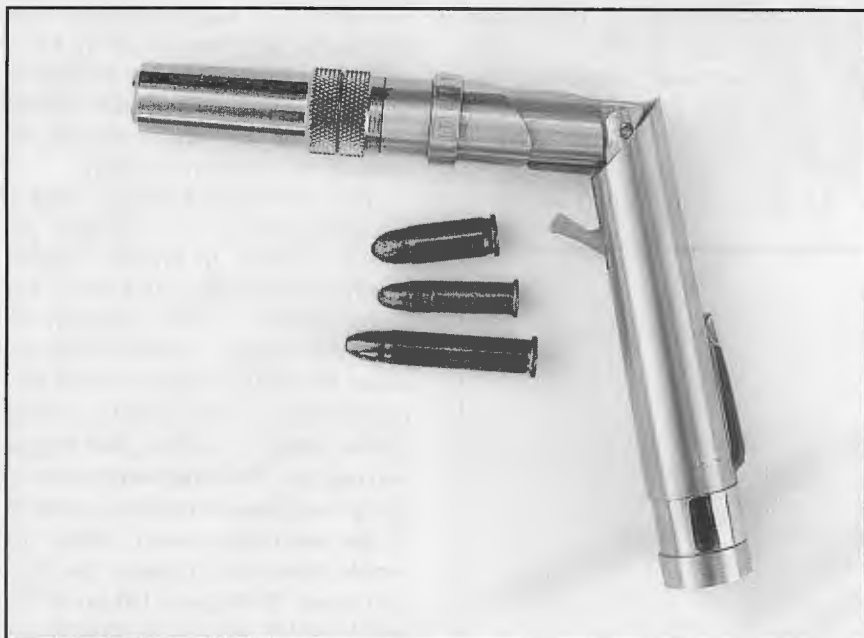
Stinger Pen Pistol in its firing configuration with the three cartridges for which it is chambered: semi-rimmed .25 ACP (6.35mm), .22 LR rimfire and .22 Magnum rimfire.
